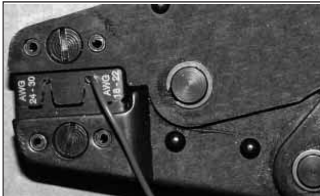
(3) The stripped wire is placed into the terminal and crimped. Note the wire's insulation must stop just short of the conductor tabs (detail)
